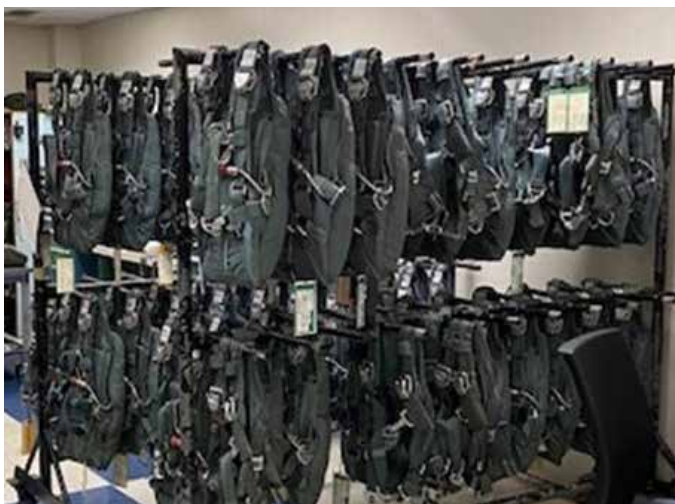
AFE is responsible for the inspection and rigging of back style automatic emergency parachutes for personnel emergency egress. (courtesy photo)
