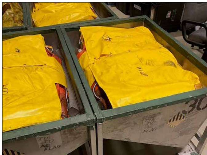
Twenty-man life rafts and survival accessory kits recently inspected and packed by AFE. Shown in containers ready to install into the wings of our newly gained C-130 H3s. (courtesy photo)
