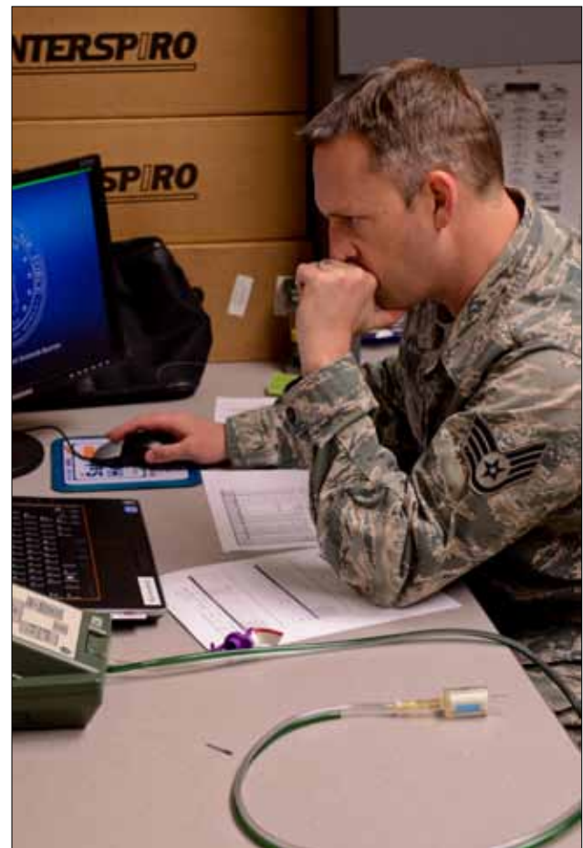
The protection assessment test instrument is used to measure the amount of particulates in the surrounding environment and compares it to the air inside the mask. It is the primary tool that the team uses to perform what they call a ‘confidence check.’
