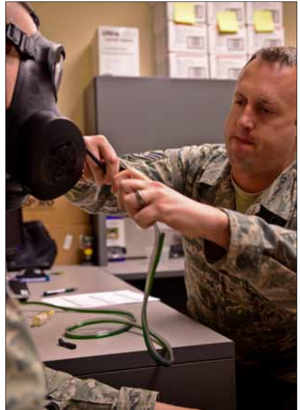
Staff Sgt. Jeffery Fancher, bio-environmental engineering technician, connects the protection assessment test instrument to the M-50 mask with an adapter before testing.
