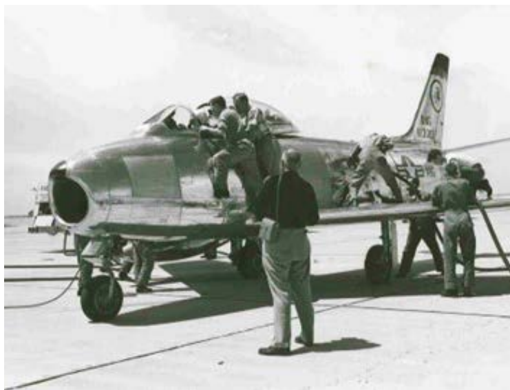
Cindee Lind 7th is refueled with engine running, during a pit stop at the Ricks Trophy Race in 1956. Note the high polish, a single drop tank, and the faired-over gun ports to reduce aerodynamic drag and increase air speed. Pilot David McCallister took first place in the 1956 race across the United States. (Courtesy of the Delaware Military Heritage and Education Foundation.)
